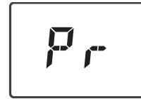
Once the final weekday has been confirmed with the  $\text{Mode}$  key, **Pr** is shown on the display.
