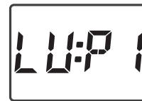
Use the  $\oplus$  or  $\ominus$  keys to assign the desired program to each weekday one after the other and confirm with the  $\text{Mode}$  key.
