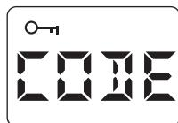
Press the  $\oplus$  and  $\ominus$  keys simultaneously for 10 s until **CODE** is displayed.
