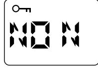
If the code was entered incorrectly, **NON** flashes. The symbol does not disappear.
